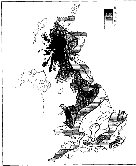
Runoff in Britain for 1975-6 expressed as a percentage of mean annual runoff (from an original diagram in Ward, 1981).
